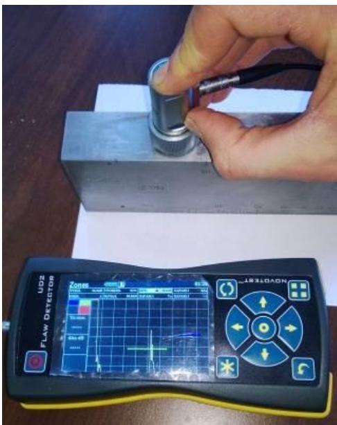
Display of the device can be operated in any orientation. There are 4 options for display orientation. This allows to customize instrument for both left handed and right handed users. Instrument can be operated in both portrait and landscape orientations.
