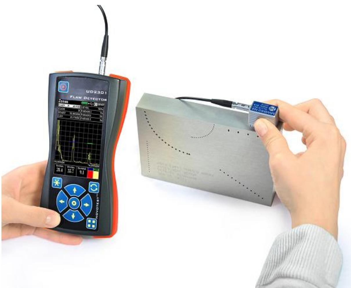
Ultrasonic flaw detector UD2301 is designed for nondestructive testing of metals, plastics, glass, composite materials, weld inspection and measurement of the thickness of the various structures.
